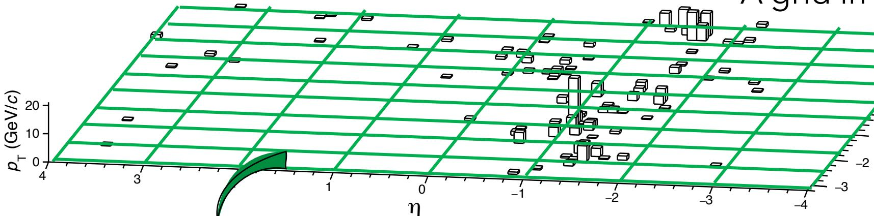
In the cell  $i$ , the charged particle multiplicity is computed:  $N_{\text{ch}}^{\text{cell},i}$
