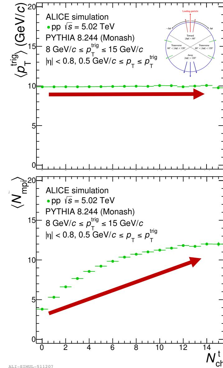
$N_{\text{ch}}^{\text{t}}$ : multiplicity in the transvere region of the di-hadron correlations at the plateau (i.e., the  $p_T^{\text{trig}}$ -region where the average UE activity saturates,  $p_T^{\text{trig}} > 5 \text{ GeV}/c$ )
